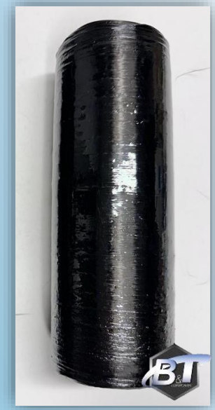
Composite specimen manufactured with Filament Winding
